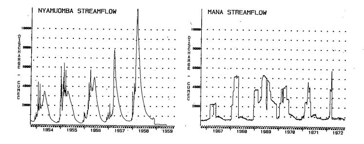
Fig. 1 The natural streamflow regime of the Zambezi River during the five years leading up to the closure of Kariba Dam. Cumec = cubic metres per second. The record flood at Victoria Falls, in March 1958, coincided with high lower catchment runoff and was gauged at Nyamuomba at 15 200 cumec.
